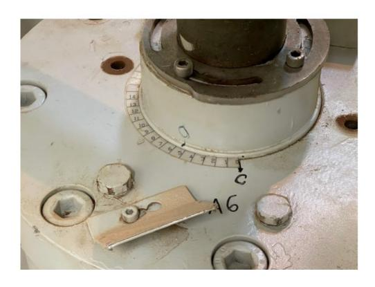
You will see that the valve location is only at the 5.5 marker which is only 37% open. Looking at the NRV design and operating position,
